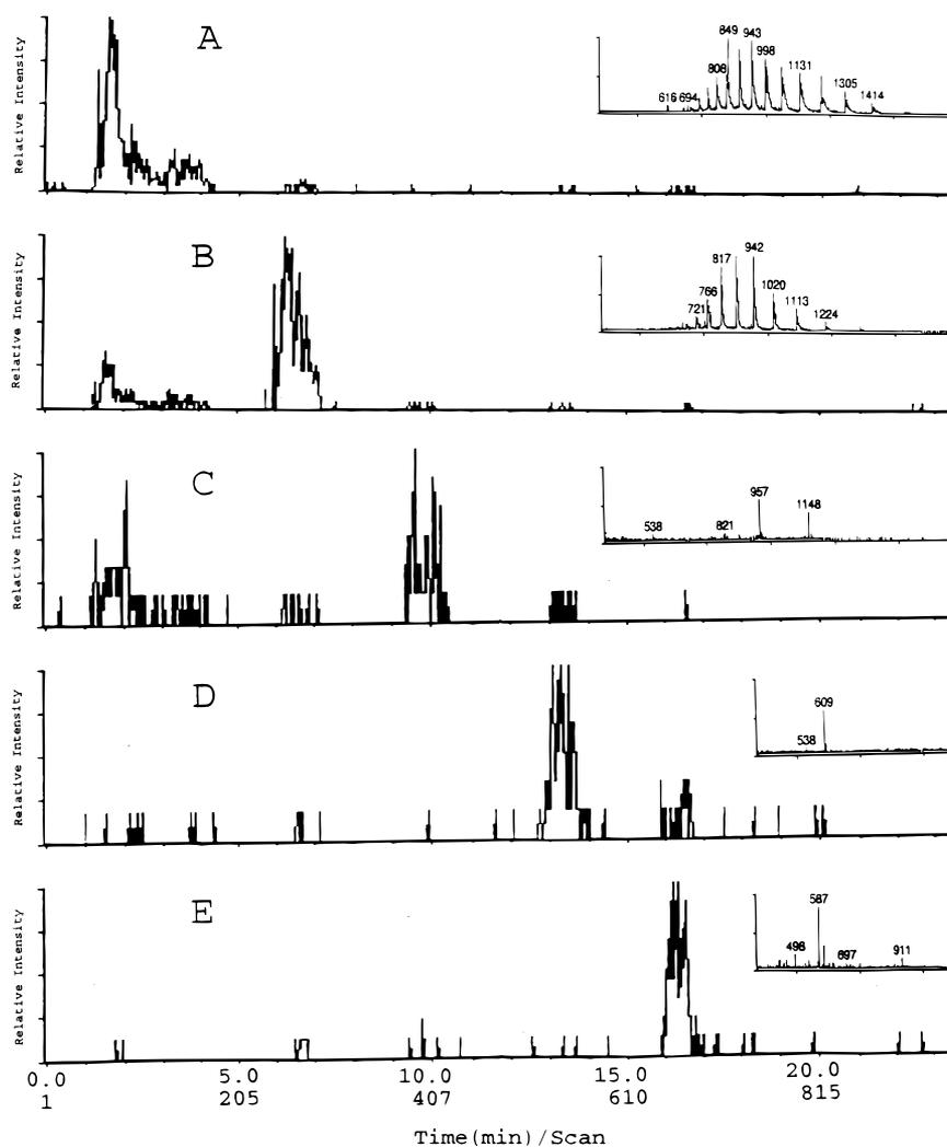
**Figure 2.** Mass chromatograms of five biomolecules, (A) myoglobin, (B) cytochrome *c*, (C) insulin, (D) reserpine and (E) renin, obtained by coupling the HPLC effluent to the 16-channel ESMS system. Each sample solution (20  $\mu$ l) was flow injected at 3 min intervals. The solution was delivered to the ES source by an HPLC pump at a flow-rate of 0.3 ml min<sup>-1</sup>. The inset in each mass chromatogram shows the ES mass spectrum of the analyte recorded.
