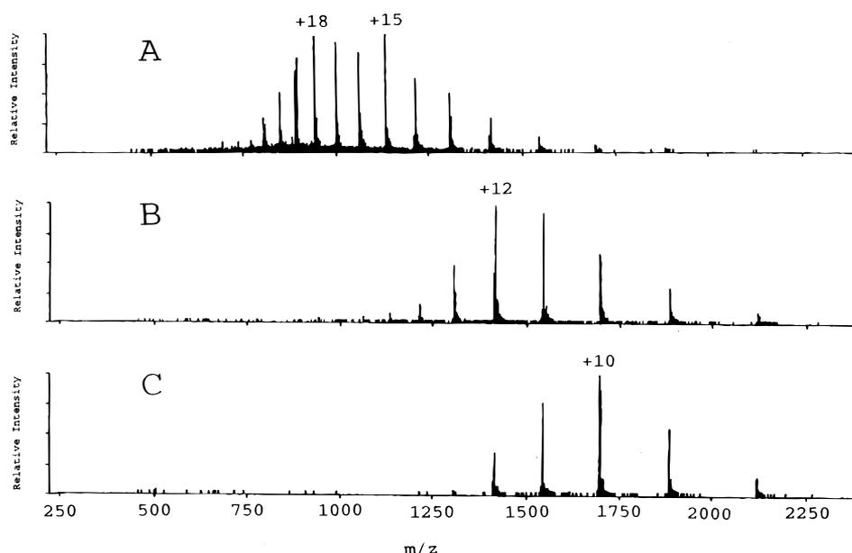
**Figure 3.** Positive ES mass spectra of myoglobin obtained by simultaneously electrospraying solutions containing denatured myoglobin molecule and diethanolamine (DEA) by the seven-channel ES source. Concentration of DEA (in methanol) in the solution: (A) 0, (B) 0.5 and (C) 1 mM.
