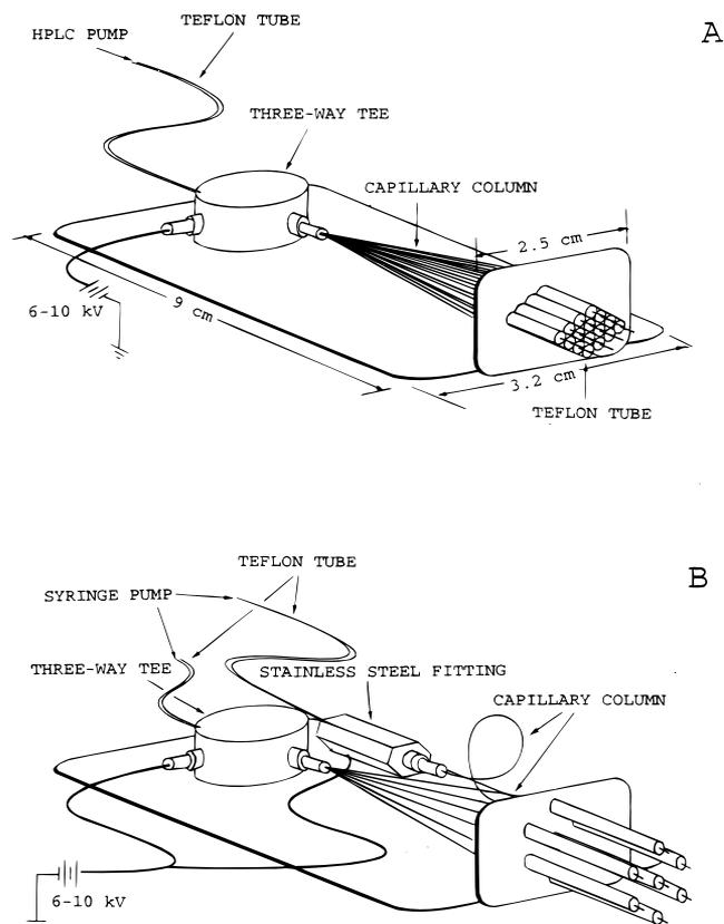
**Figure 1.** Schematic diagrams of (A) the 16-channel and (B) the seven-channel electrospray ionization source.
